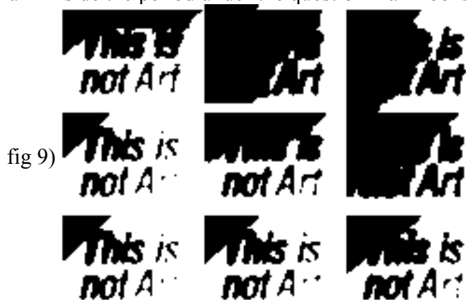
This is it at full resolution.. You can see how the pattern is thinned or fattened to create the gray shades needed...
